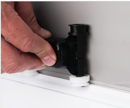
900 µm Clear Fiber into ILU Fiber Pathway with ILU Installation Tool
