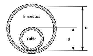
$$Fill Ratio(\%) = \frac{Outer \ Diameter \ of \ Cable \ (d)}{Inner \ Diameter \ of \ Duct \ (D)} \times 100$$
