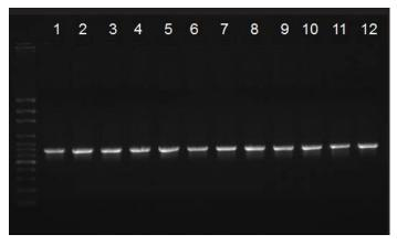
**Figure 1. Representative Gel of PCR product.** The post-PCR GFP DNA from each replicate was loaded onto a 1% agarose gel in an electrophoresis unit. Images of the resulting gels were used for the quantification of the PCR product concentration. One band representing the amplified GFP DNA was seen after using Axygen single PCR tubes (lanes 10-12), Competitor A (lanes 7-9), Competitor B (lanes 4-6), and Competitor C (lanes 1-3).
