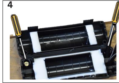
Drill the screw holes on the cover and body.
