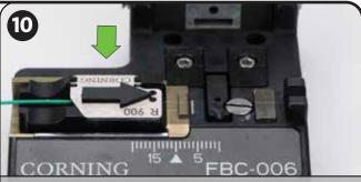
Place Holder in Cleaver and Slide to the Right Until It Hits the Positive Stop
