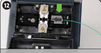
Load the Fiber Holder into the Splicer (on the Right Side)
