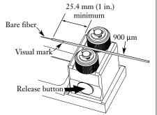
Insert the fiber into the lead in tube. The visual mark on the fiber must be within 2 mm of the lead in tube.
