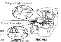
For the FBC-001 cleaver: position the marks so that the buffer coating lines up with the fiber guide's stop and the end of the fiber is secured under the spring-loaded fiber clamp. Press down the cleaver arm until it touches the fiber guide. This will "score" the fiber. Only light pressure is necessary. Release the cleaver arm, then gently flex the fiber guide to break the fiber. If the fiber guide is flexed excessively to break the fiber, a poor cleave will result.
