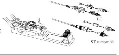
Slide the strain relief boot onto the fiber/cable. For LC connectors slide the boot on, then slide the trigger on.
