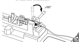
Rotate the crimp handle 180° until it contacts the lead in tube. Push the handle down firmly and lift it back up.
