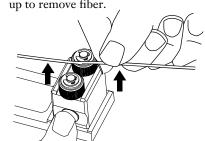
Move the slider handle back and lift out the connector.
