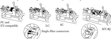
**CTS Installations:** Remove the clear ferrule dust cap on all connectors. For LC and ST-compatible connectors, also remove the black load adapter.
