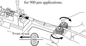
Rotate the wrench handle down 90° to cam the connector.
