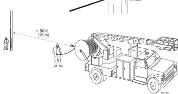
**6.4.** Pull off the necessary amount of slack as specified in Step 4.8. Prepare the cable and install the deadend as specified in Section 8.
