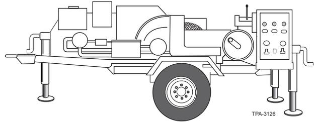
**NOTE:** Carefully select equipment that maintains bend radius. Not all outside plant equipment is well-suited for fiber optic cable installation.
