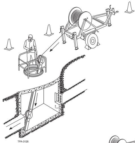
**Step 2:** Unreel the remaining cable in a figure-eight configuration.
