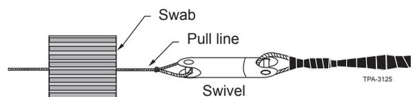
Additional lubricant should be added before bends and known severe offsets and sections with "uphill" elevation changes.
