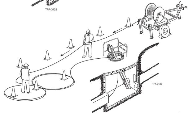
**Step 4:** Pull the exposed end of the cable in the opposite direction to complete the pull. Hand tending of the cable paying off from the figure-eight coil is normally required.
