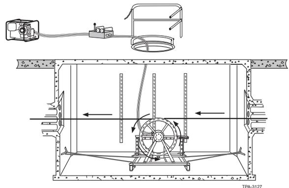
Use of multiple winches requires compatible pulling equipment and careful coordination of winch speeds. Consult the equipment manufacturer's instructions for necessary details.
