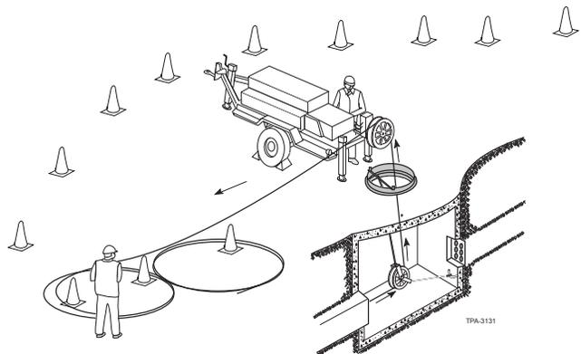
**Step 2:** After the pulling eye is connected to the next section of the pull-line, feed the cable by hand back into the manhole and pull it to its next destination. The cable may be pulled directly from a figure-eight by a winch, provided the capstan or sheave used at the entry manhole ensures sufficient bend radius. Hand tending of cable paying off from figure-eights is normally required.
