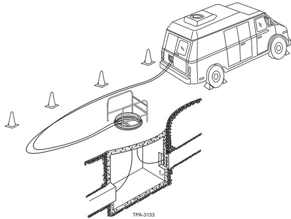
**Step 10:** Once the cable is pulled into place and appropriate slack is available at splice or termination points, begin securing all the innerduct to cable racks on the manhole walls. Begin racking at the center manhole and proceed to the end manholes. Maintain the cable's specific minimum bend radius.
