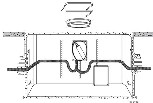
**Step 14:** Fiber optic warning signs should be placed on all innerduct containing fiber optic cable. Warning signs can help prevent damage resulting from the cable being mistaken for something else.
