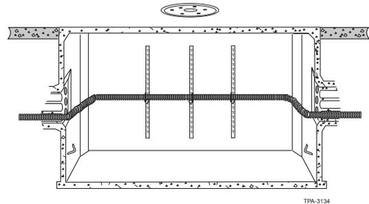
**Step 13:** Store coiled splicing slack in the splicing manholes so that it is not likely to be damaged during later work in the manhole. If possible, store the slack in an enclosure designed to store splicing slack and a splice closure. Place an end cap on any bare cable ends to prevent moisture or dirt intrusion.
