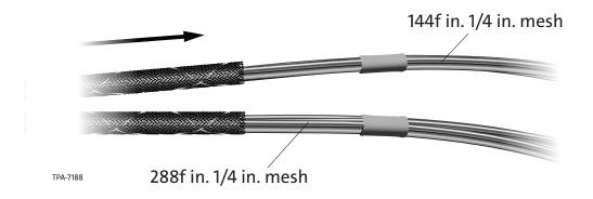
**Step 5:** Apply one wrap of electrical tape 1.25 inches from the end of the subunit sheath.
