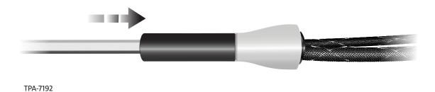
**Step 2:** Place a mark on the subunit where the heat shrink stops.
