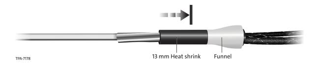
**Step 8:** Shrink the heat shrink and tear off the remaining foil flush to the end of the heat shrink.
