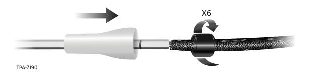
**Step 7:** Slide the funnel up to the mesh. The funnel should stop at the 1 inch mark on the subunit sheath.
