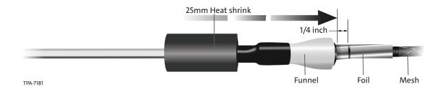
**Step 11:** Install the 25 mm heat shrink to the mark and shrink the heat shrink.
