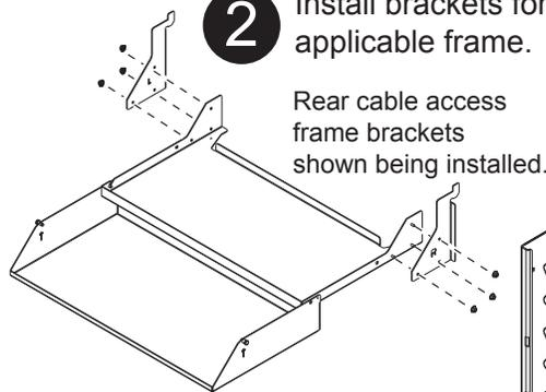
Rear cable access frame brackets shown being installed.
