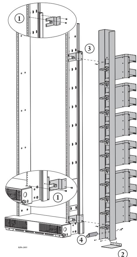
Figure 1 — Attach IBU to FMS Frame
