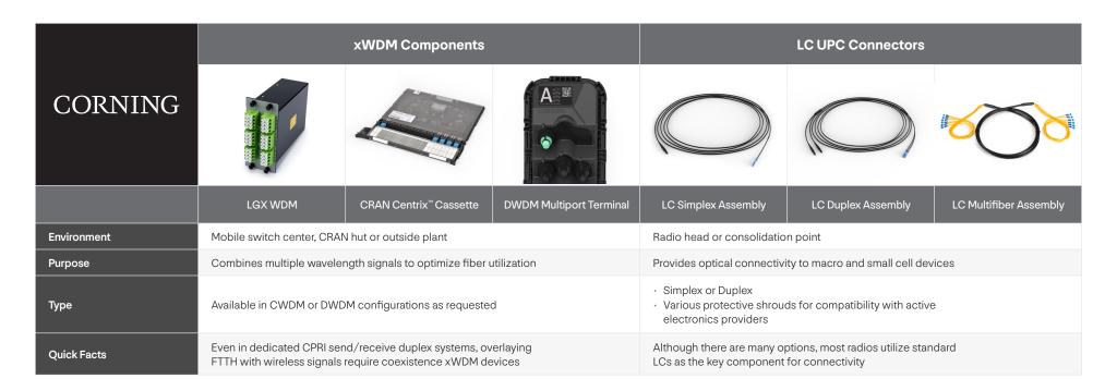
xWDM devices and LC connectors are key enabling components that allow for convergence of an existing FTTP network with wireless capability. The fundamental infrastructure components otherwise remain the same and can be found elsewhere in this guide.
