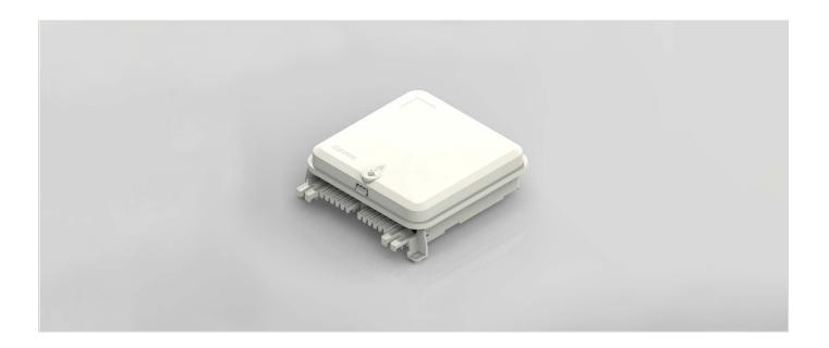
This Optical Access Point (OAP) is designed for aerial distribution application. Part of the PBO range, it can connect to 12 customer cables/drops, 1 distribution cable (mid-span) and 2 secondary distribution cables. Its organizer is compatible with both G.652.D and G.657 fibers, loose tubes and micromodules. It can be equipped with standard trays from the BPEO product range. The organizer can receive four 1-slot trays (monozone) or two 2-slots trays (bizone).
