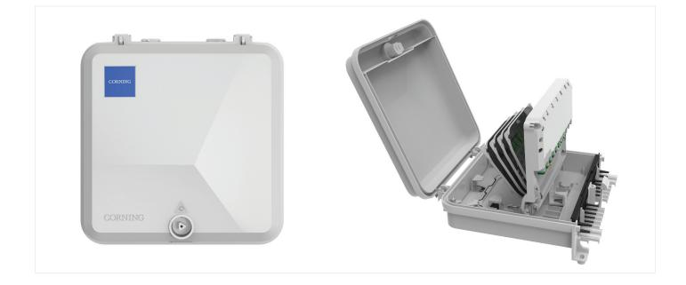
This Optical Access Point (OAP) is designed for aerial distribution applications. This Distribution Terminal is part of the PBO range and can connect to 10 customer cables/drops, 1 distribution cable (mid-span) and 2 secondary distribution cables. Its organizer is compatible with both G.652.D and G.657 fibers, loose tube and micromodules. It can be equipped with standard trays from the BPEO product range. The organizer can receive 1-slot trays (5 mm) or 2-slot trays (10 mm).
