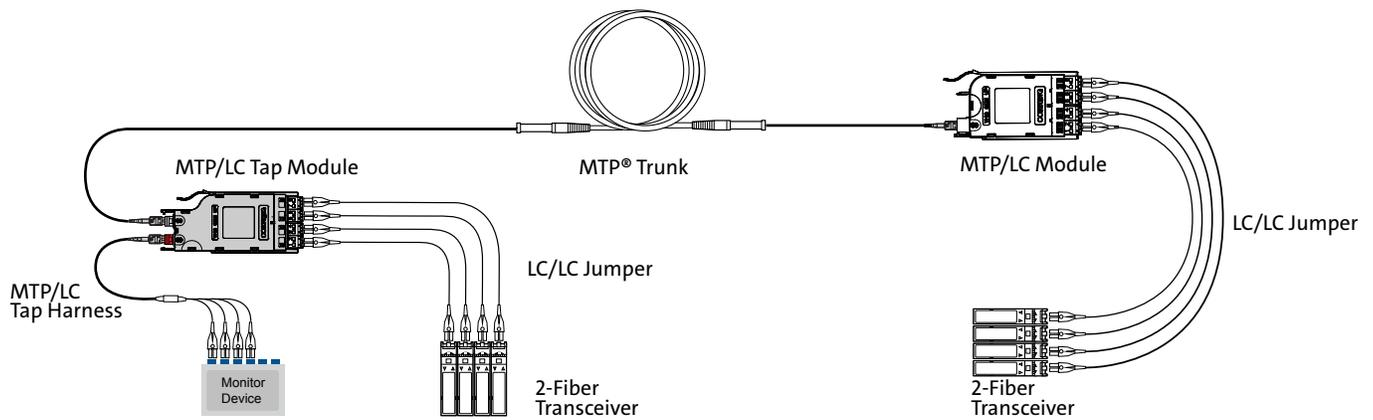
In the above scenario, the configuration B EDGE tap module is deployed as an integrated part of the structured cabling system to support serial duplex transmission. Within the system, the tap module functions like a normal Universal-wired module, while also sending the split signal to the MTP TAP port. This deployment eliminates the use of extra rack space and maximizes the channel reach by reducing the number of loss components in the system.
