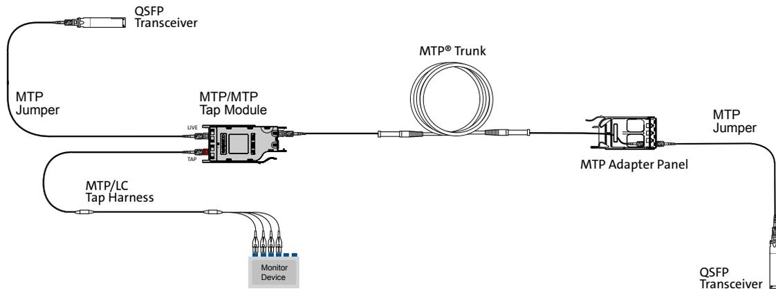
When migrating from duplex transmission to higher data rate via parallel transmission such as 40G, MTP equipment connectivity is required. The above scenario depicts the use of an EDGE8 Configuration C tap module for a parallel transmission system. A MTP jumper is used to interconnect the MTP parallel link equipment port to the MTP LIVE port in front of the tap module. When the monitoring equipment can receive a parallel input, a MTP/MTP tap harness is used to interconnect to the monitor device.
