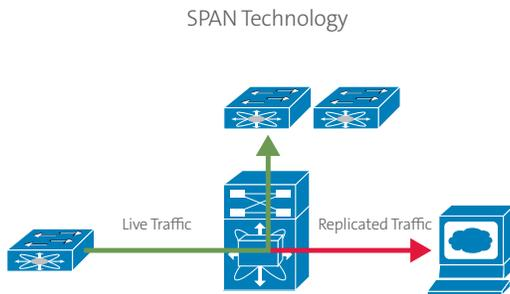
**Active data extraction**, typically called switch port analysis (SPAN) or port mirroring, uses an electronic device (usually a switch) to replicate, or mirror, the link’s data and send it to a monitoring device.
