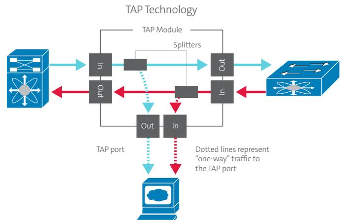
**Port tapping**, which is completely passive, extracts the data via a device that can split signals from both directions between its intended recipients as well as a monitoring device.
