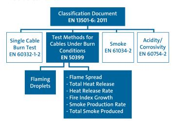
Note: bunched test does not appear in the diagram above, but tests according to EN 50399 are conducted in a bunched configuration
