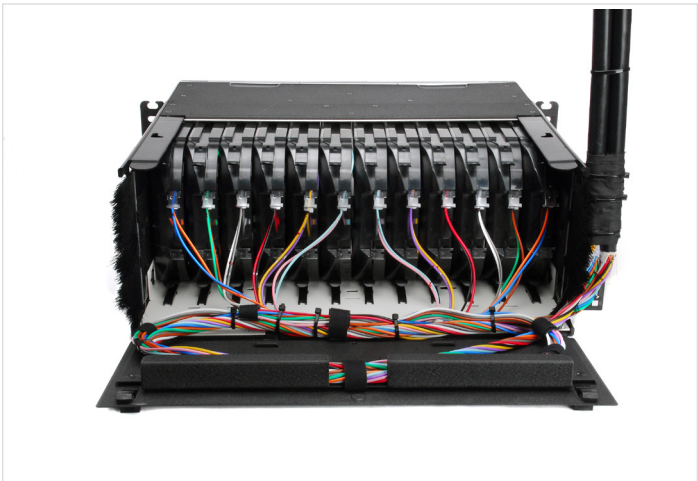
CCH-04U Closet Connector Housings pictured open | Photo LAN2555
