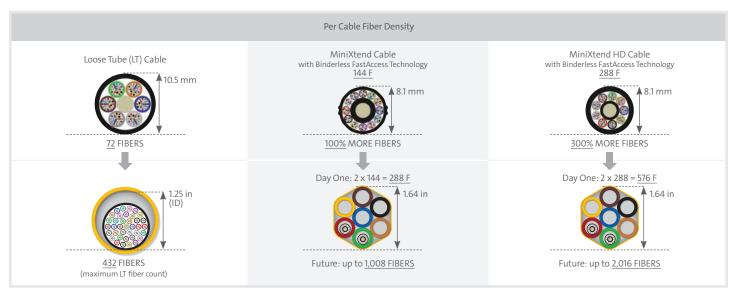
\*Corning's proprietary Binderless\* FastAccess® technology refers to the combination of a Corning FastAccess technology jacket with an innovative technology used to bind cable construction through the manufacturing process, eliminating the use of binder yarns and waterblocking tapes.
