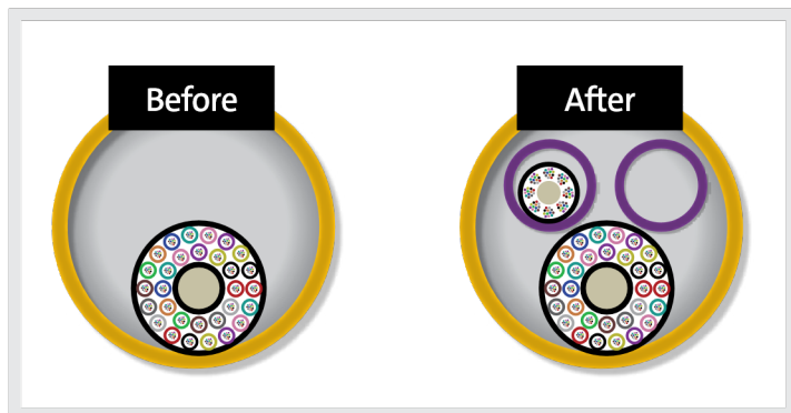
Figure 32. Before and After of an Existing Duct With a Cable Installed and Two New Microducts Installed
