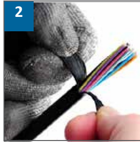
Figure 13. Cable Jacket Then Simply Pulled Apart to Required Stripping Length
