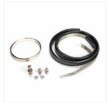
Bonding and Grounding Kit This kit is used for maintaining internal shield continuity and external grounding. A pressure valve provides for external flash testing and pressurization.
