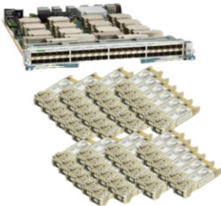
Figure 4. 36x40G QSFP line card.
