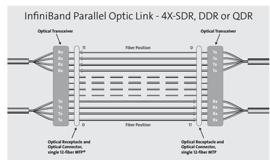
and the other 10 to receive 10 Gb. Thankfully, in 2015 the IEEE ratified 100G-SR4 transmitting 25 Gb over 4 fibers and receiving 25 Gb over the other 4 fibers to reach our aggregated 100 Gb speed using the same 8-fiber platform as 40GBASE-SR4, and this consistency of fiber counts and electrical lanes continues as we move toward 200G and ultimately the 400G we saw announced last year.
