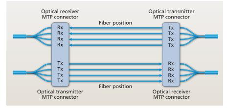
40GBase-SR4 employs eight-fiber parallel transmission. In this setup, four fibers each transmit 10G, and a different four fibers each receive 10G. The MTP is the defined connector interface into the transceiver.
