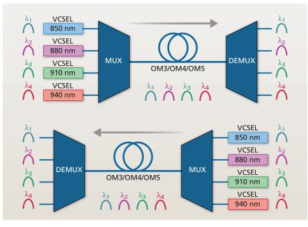
A two-fiber, 40G short wave division multiplexed (SWDM) transmission system operates over four wavelengths per fiber across the range from 850 to 940 nm. One fiber is dedicated for transmit and the other is dedicated for receive.
