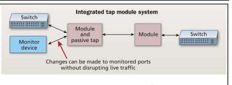
An integrated tap module allows administrators to perform moves, adds, and changes to monitored ports without disrupting the live network. This can save as much as eight hours in downtime annually.
