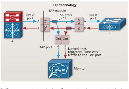
Traffic access port—tap—technology allows non-intrusive access to data flowing across the network and enables monitoring of network links. A tap uses passive optical splitting to transmit inline traffic to an attached monitoring device without data-stream interference.
