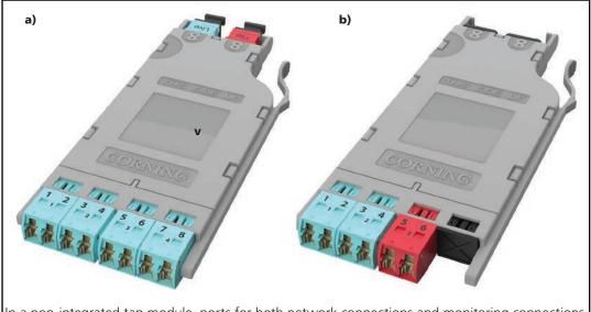
In a non-integrated tap module, ports for both network connections and monitoring connections are exposed. In integrated taps, only the network ports are exposed; the monitoring ports are connected on the system backplane.
