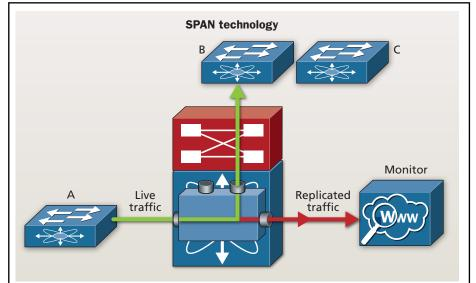
Switched port analyzer—SPAN—is also known as port mirroring. A SPAN port copies traffic from any port to a single unused port, and prohibits bidirectional traffic to protect against traffic backflow into the network. The SPAN port directs packets from its switch or router to the test device for analysis.
