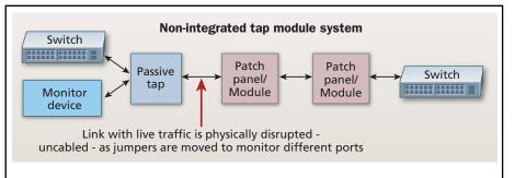
A non-integrated tap module is deployed as a standalone device outside the structured cabling networks. Traditionally with non-integrated taps, when an administrator needs to change monitored ports, the link must be disabled temporarily.
