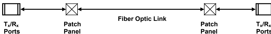
Figure 1: Fiber Optic Link Schematic
