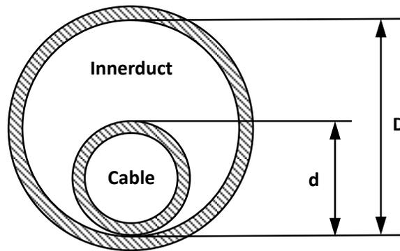
$$\text{Fill Ratio (\%)} = \frac{\text{Outer Diameter of Cable (d)}}{\text{Inner Diameter of Duct (D)}} \times 100$$
