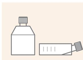
**Rectangular flasks** have a ramp from the bottom to the canted neck for easier pouring and pipet access. Most canted neck flasks also have an anti-tip skirt to enhance stability.
