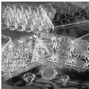
Permeable supports, also known as cell culture inserts, are an essential tool for the study of both anchorage-dependent and independent cell lines.
