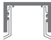
**Phenolic-style caps** are designed (when loosened) for use in open systems requiring gas exchange. With the caps slightly loosened, gas is exchanged between the environments inside and outside of the flask.
