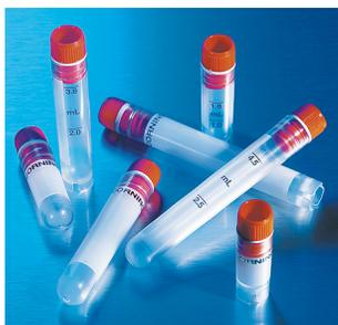
Internal thread color cap cryogenic vials
