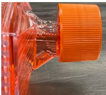
Figure 4. Cap should be tightened to a torque of 18 lb-in/2 nm. All threads should be covered by the cap. Placing the flask on end in the incubator and then lowering it slowly will keep any bubbles in the cap area.
