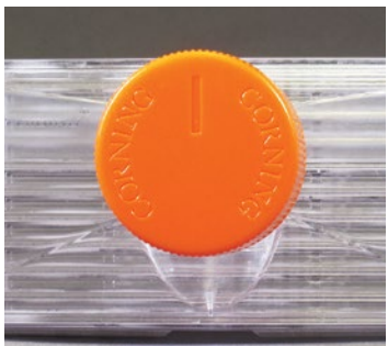
Figure 2. Venting position to be used when pre-warming Corning® HYPERFlask® and HYPERFlask M vessels when the vessel is empty or contains low volumes of liquid for prolonged periods of time (greater than 60 minutes).
