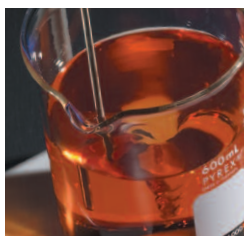
Temperature Probe for precision liquid temperature control in the liquid (as opposed to the plate top)
