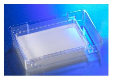
Transwell large format inserts feature a two-tier receiver tray, which permits submerged or air-liquid interface (ALI) culture.
