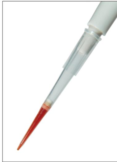
Axygen GEN3 multi-barrier pipet tips seal on contact with liquids and prevent liquids or aerosols from passing through, reducing cross-contamination.
