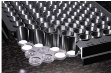
Figure 1. FiltrEX 96 well filter plate design Proprietary nozzle design and individually integrally sealed filter disks prevents filtrate cross contamination. Rigid design and wide skirt allows for robotic handling and bar coding. US Patent 6,391,241
