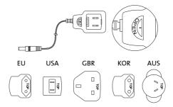
To mount the adapter, it should be inserted into the slots of the housing in the direction of the arrow, until you hear a click.
