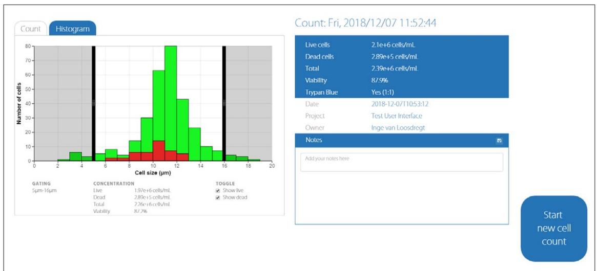
**Figure 6.** Example of gating the histograms. The cells that are in the shaded regions are excluded from the cell count. The cell concentrations and viability corresponding to the gated histograms are displayed underneath the histograms.
