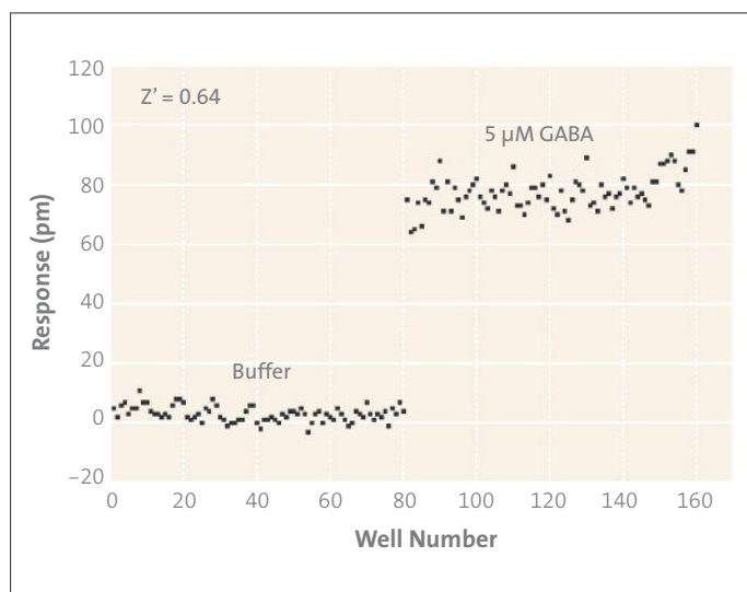
Figure 4. GABA A assays on the Epic System are very robust. Assay robustness was evaluated using an EC 80 dose of GABA, and the peak response plotted using GraphPad Prism® software (n= 80 wells). The experiment was performed in triplicate and each time the Z' exceeded 0.6.
