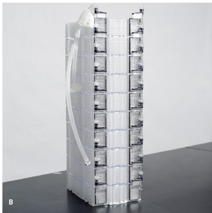
Figure 1. (A) HYPERStack-12 and HYPERStack-36 Cell Culture Vessels. (B) HYPERStack-120.
