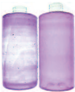
Figure 17. As these crystal violet stained roller bottles show, rotating bottles too quickly (left bottle) results in poor cell attachment and growth when compared to a bottle rotated at a slower speed (right).
