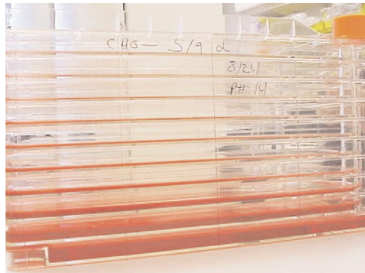
Figure 1. Top: tilting of CellSTACK® chamber to pool media in lowest layers. Bottom: Media levels after pooling into bottom layers.
