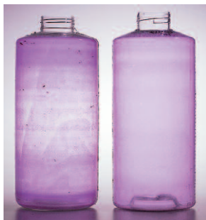
Examining the morphology of these stained roller bottles (containing MRC-5 human fibroblasts) is a good way to check if the cells are “happy”. The bottle on the left was rotated at too high a speed resulting in poor attachment and growth and very “unhappy” cells.
