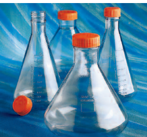
Corning® Erlenmeyer flasks are often used for growing insect cells in suspension.
