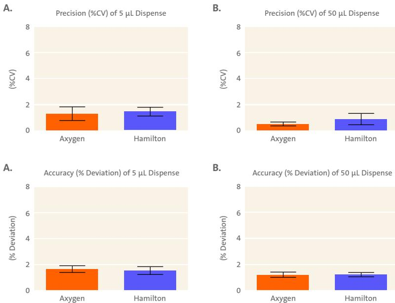
**Figure 1. Precision (% CV) analysis of 50 µL tips.** The % CV of Axygen and Hamilton 50 µL tips dispensing (A) 5 µL and (B) 50 µL using the Microlab STAR liquid handler was determined using the Artel MVS® System. There was no significant difference in % CV between each brand. Data shown with standard deviation (SD). n = 48.
