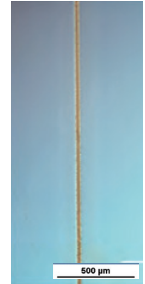
Gorilla® Glass 3 (7 Newton Load)
