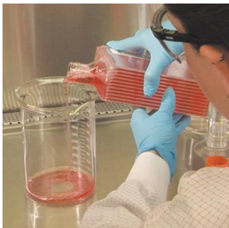
Figure 5. This initial pouring position allows medium to flow over the air dam and reduces foaming.
