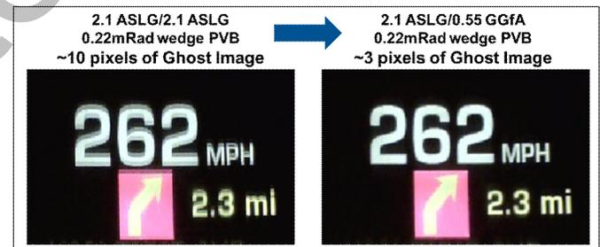
Figure 16. Images showing the improved HUD quality with the GGfA windshield design.
