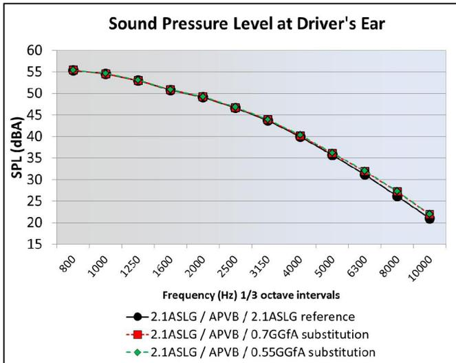
Figure 11. In-vehicle sound pressure level for lightweight windshields and standard reference (modeling results, wind noise).
