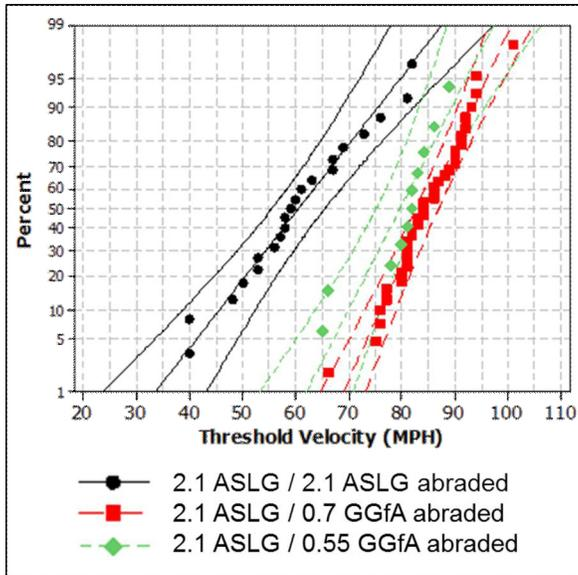
Figure 8. Ball bearing test results (45° incident angle, 1g ball bearing, Weibull with 95% confidence interval).
