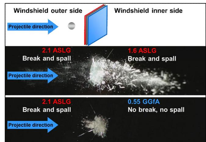
Figure 10. Photographs of high speed ball bearing windshield impact of two laminate constructions (1 gram, ¼ inch diameter projectile, 120 mph, 90° incidence angle).
