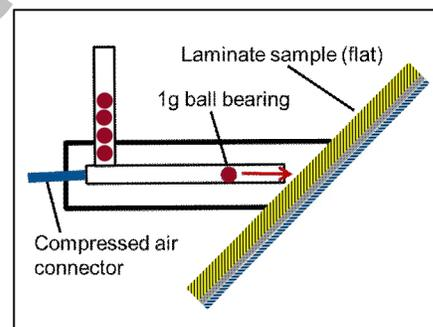
Figure 7. Ball bearing test apparatus (schematic).
