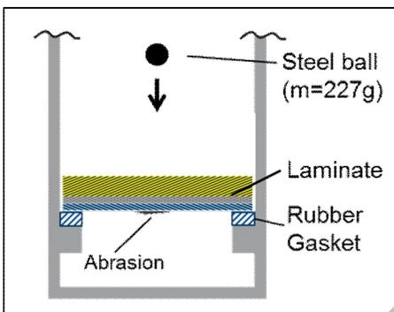
Figure 5. Ball drop test schematic (not to scale).
