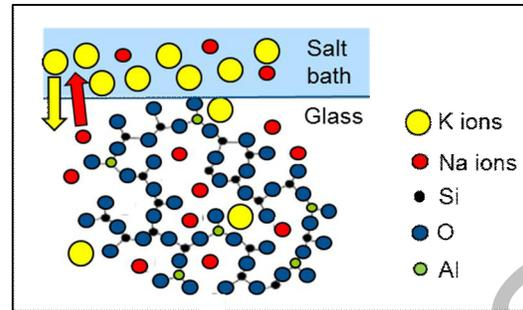
Figure 2. A schematic of the GGfA ion-exchange process.
