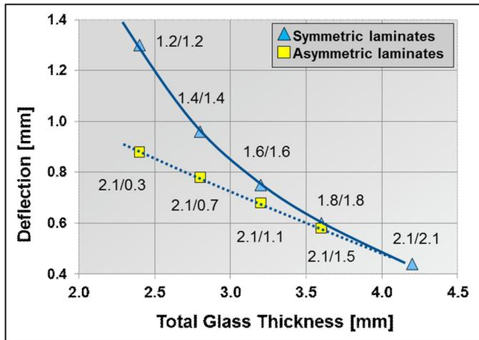
Figure 14. Modeling results for deflection for symmetric and asymmetric laminates (Ball-on-frame case).
