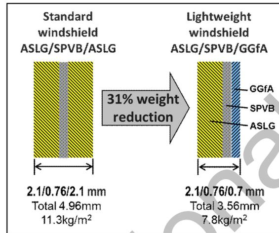
Figure 4. Standard and proposed lightweight windshield construction.
