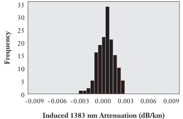
The above data clearly shows the resistance of Corning’s ITU-T G.652.D fiber to increases in 1383 nm attenuation upon exposure to hydrogen. This industry-leading performance allows Corning’s G.652.D product offerings to perform reliably not only in the O-, S-, C- and L-bands, but in the E-band as well, which gives operators a significant increase in channel capacity.
