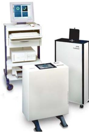
*The FlatMaster series offers the capability to measure parts that range in size from 5-200 mm. Each system comes with an interferometer (two versions shown here) and a Windows-based PC with Corning Tropel TMS software.*
