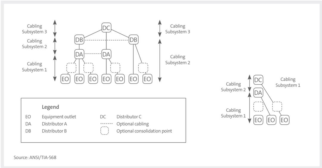
**2. Determine the location of the MC/DC, IC/DB, and HC/DA**
