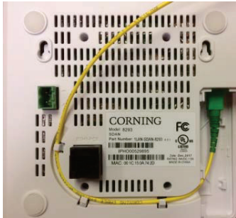
Figure 6 Fiber routing guide
