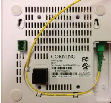
Figure 3 Fiber routing guide
