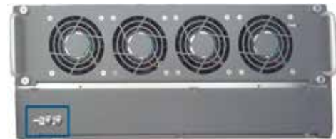
Figure 6. Location of Chassis Grounding Lug
