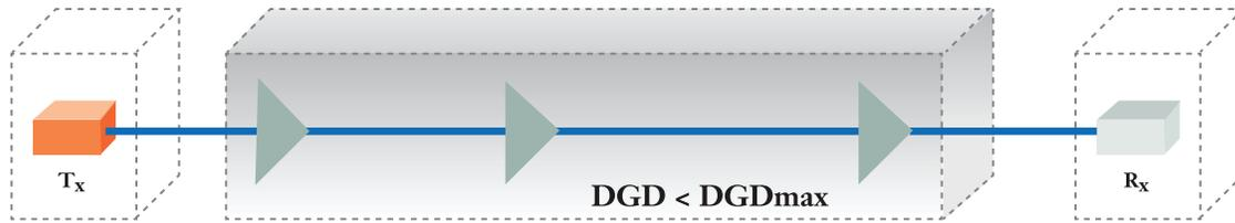
Figure 12. From Interface Point of View All Optical Path is Black Box with DGD Below Some Maximum Allowed Level DGDmax
