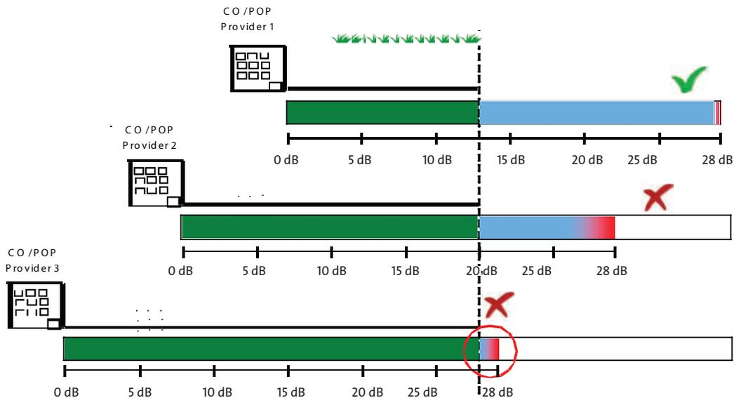
**Poor indoor cabling can lead to excessive consumption of power budget within the building, precluding competitive providers, located more distance from that building from offering service to the subscriber. Indoor cabling power loss must be controlled and minimized to ensure competitive open access to subscribers.**
