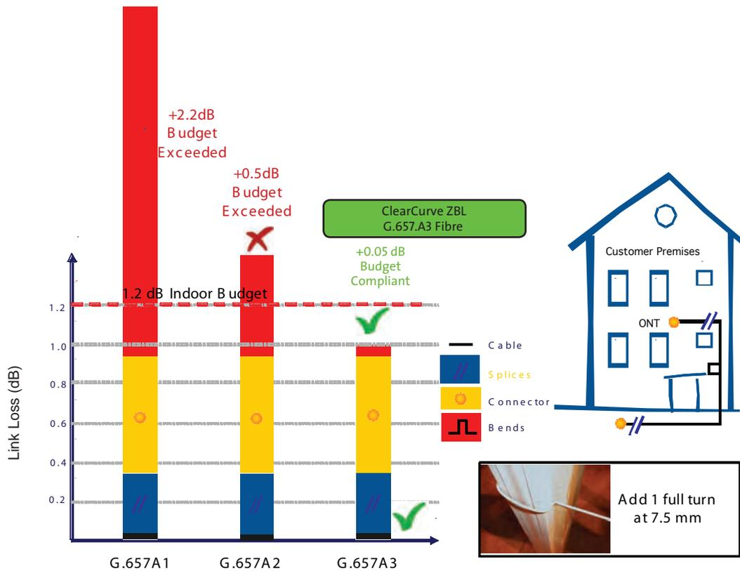
Only G.657.A3/B3, the truly bend insensitive fibres, can effectively give us near zero bend loss and so ensure that we maintain very low indoor cabling loss to achieve compliance with the indoor cabling standards.
