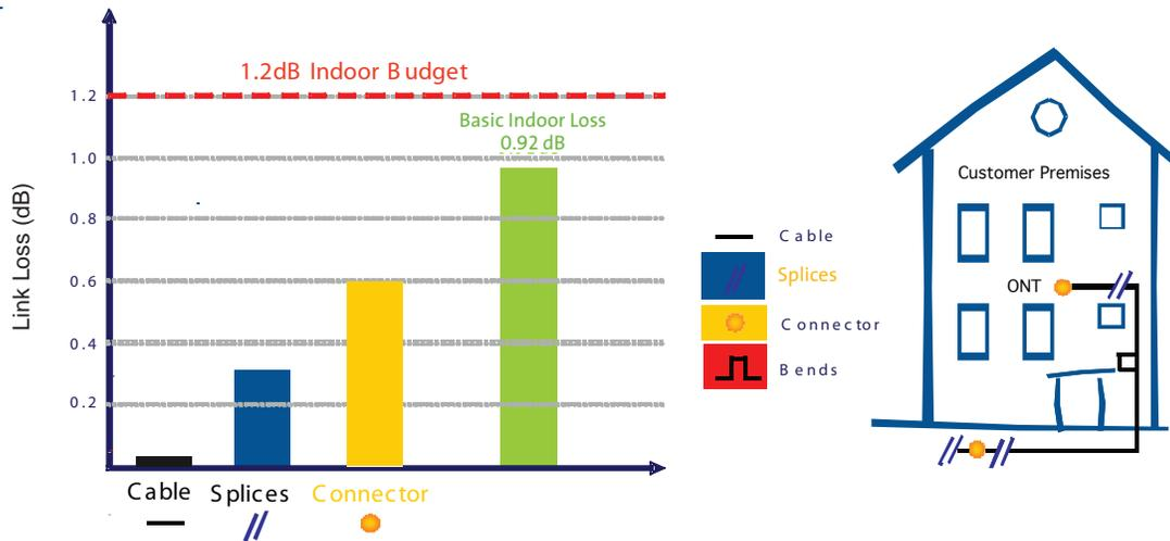
**New indoor power budgets are readily consumed by a basic installation involving 50 m of cable, three splices and two connectors. Little headroom is available for signal loss due to bends.**
